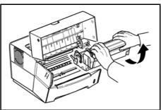
3 Using the green handles lift the *Drum Unit* out of the machine.
